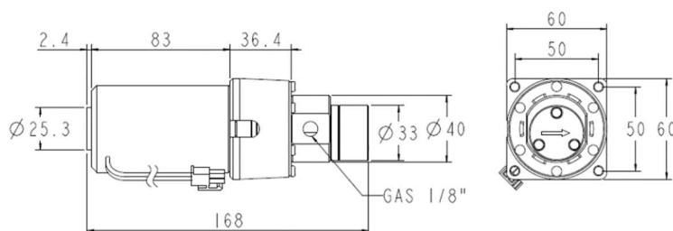
400 series available in 24VDC motor drives allows simple control by varying the voltage on different performance.
